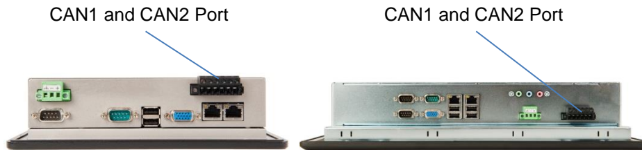
Figure 6.1 – CAN1 & CAN2 Connector Locations ZX452 (Left) and ZX752/1152 (Right)
